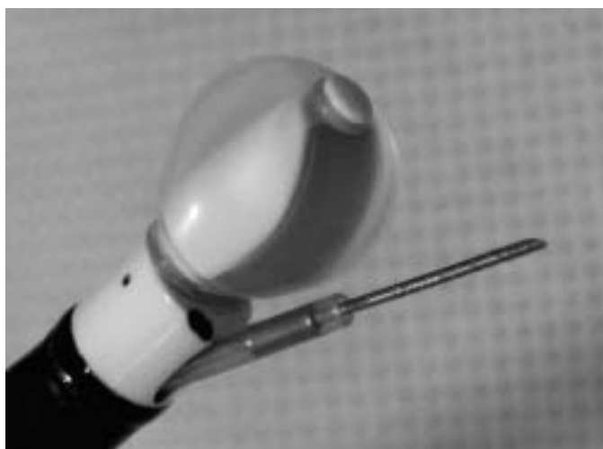
FIGURE 1. Distal end of the endobronchial ultrasound probe (XBF-UC260F-OL8; Olympus Ltd, Tokyo, Japan), showing the curved-array ultrasound transducer with the balloon inflated and a 22-gauge aspiration needle protruding from the biopsy channel.
