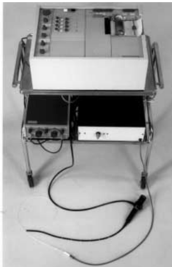
Fig. 1. — The recording unit with fibreoptic bronchoscope and the glass fibre cable, light source, filter and ink jet writer.
