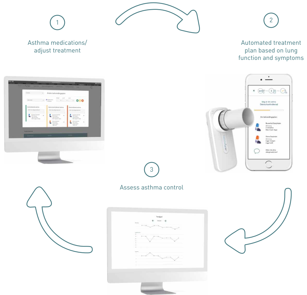
FIGURE 2 AsthmaTuner is a certified (CE-marked) electronic clinical decision support system with cloud-based data storage, a healthcare interface and a downloadable patient app (Android or iOS). The intended use of AsthmaTuner is to automate asthma self-management by letting healthcare providers prescribe treatment and patients register symptoms and measure forced expiratory volume in 1 s with a Bluetooth spirometer. The patient then receives immediate feedback on asthma control and an image of the correct inhaler(s) to use and the dose. The healthcare provider can simultaneously monitor the patient's asthma control.
