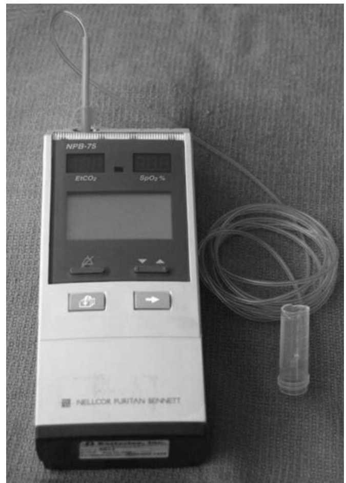
FIGURE 1. A modified sensor for detection of end-tidal carbon dioxide tension. The modified sensor is 5 cm long with a diameter of 1 cm.
